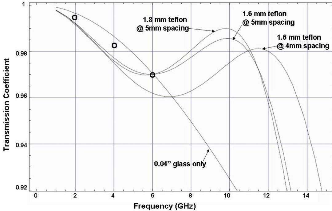
Figure 6: Transmission through the 1mm (.040") thick glass sphere and three different choices of Teflon thicknesses and separations. The three circles show the expected transmissions through the conical part of the feed with no Teflon at 2 GHz, 4 GHz, and 6GHz, where the cone and sphere thicknesses are the same.
